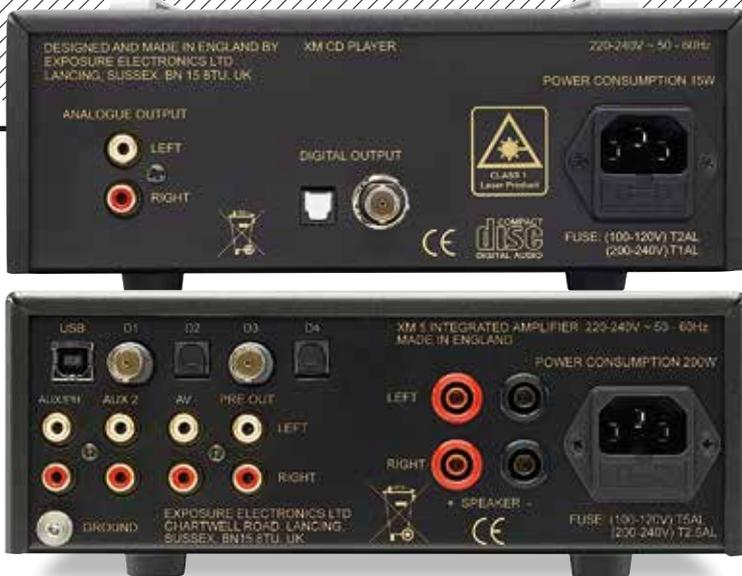
**ABOVE:** CD player [top] has fixed line (RCA) and digital (optical/BNC) outputs, but no digital ins. The amp [bottom] has two line inputs and MM phono plus USB-B and pairs of BNC/optical digital ins. Preamp out (RCA) is joined by 4mm speaker plug sockets
