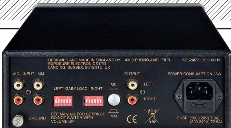
**ABOVE:** MM and MC inputs on RCAs are selected via a pushbutton while DIP switches select cartridge loading and gain from +40dB to +60dB
