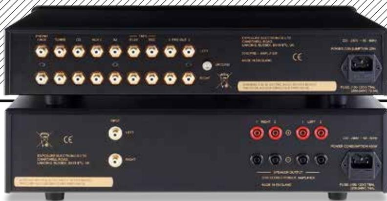
**ABOVE:** The 3510 pre [top] offers five line inputs (one for an MM/MC phono option), a tape loop and two preamp outs on RCAs. The 3510 power amp [bottom] includes RCA inputs and dual 4mm speaker cable sockets (for bi-wire applications) but are for banana plugs only, so there is no provision for bare wire or spades here
