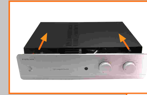
Slide the cover back about 2 cm until it is free to move upwards to reveal the main circuit board.
