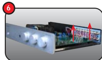
Observe the position of the plug on the phono module and carefully plug it in, ensuring that all of the pins are inserted correctly into their connectors.
