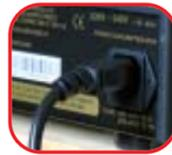
b) Connect the mains cable to the IEC mains input socket.
