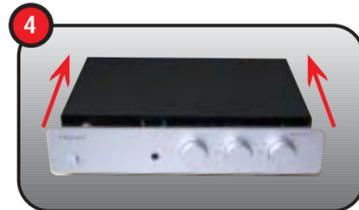
Slide the cover back about 2 cm until it is free to move upwards to reveal the main circuit board.
