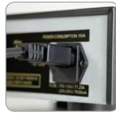
a) Connect the mains cable to the IEC mains input socket.
