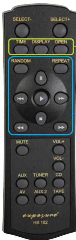
**TIME DISPLAY** Track time countdown. Press once to turn display off. The display will stay off until another button is pressed, and it will then go off again after a short delay. Press again to turn it back on.
