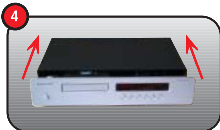
Slide the cover back about 2 cm until it is free to move upwards.
