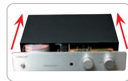
4 Slide the cover back about 2 cm until it is free to move upwards to reveal the main circuit board.
